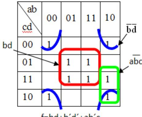
$$f = bd + \overline{b}\overline{d} + \overline{a}\overline{b}c$$
