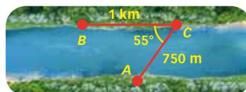
$$\begin{aligned}\overline{AB} &= \\ &= \sqrt{750^2 + 1000^2 - 2 \cdot 750 \cdot 1000 \cdot \cos 55^\circ} = \\ &= 837,94\end{aligned}$$
