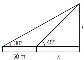
$$\begin{aligned} \operatorname{tg} 45^\circ &= \frac{h}{x} \\ \operatorname{tg} 30^\circ &= \frac{h}{50+x} \end{aligned} \quad \left. \begin{array}{l} h=x \\ \hline \end{array} \right. \\ \rightarrow 28,88 + 0,577x &= x \rightarrow x = 68,27 \end{aligned}$$
