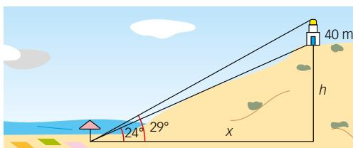
$$\begin{aligned} \operatorname{tg} 24^\circ &= \frac{h}{x} \\ \operatorname{tg} 29^\circ &= \frac{h+40}{x} \end{aligned} \quad \left. \begin{array}{l} h=0,445x \\ \hline \end{array} \right. \\ \rightarrow 0,544x &= 0,445x + 40 \rightarrow \\ \rightarrow x &= 404,04 \rightarrow h = 179,8 \end{aligned}$$
