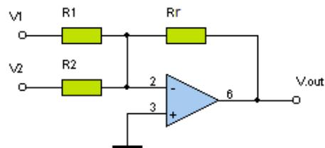
$$-V_{out} = A_V * (V_1 + V_2)$$
