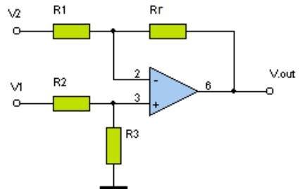
$$V_{out} = A_V * (V_1 - V_2)$$
