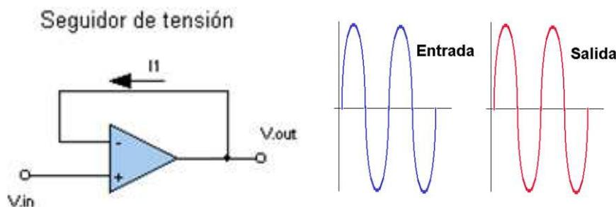
$$A_V = 1 + \frac{R_f}{R_1} \quad R_1 = \infty; R_r = 0 \Rightarrow A_V = 1$$
