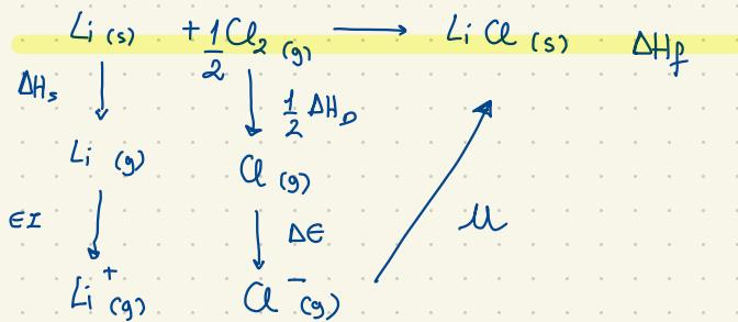
$$\begin{aligned}\Delta H_f \text{ LiCl} &= \Delta H_s + \epsilon I + \frac{1}{2} \Delta H_d + \Delta E + U \\ -408,3 &= 129,3 + 520,2 + \frac{1}{2} 244 + (-349) + U \\ U &= 861 \text{ kJ/mol}\end{aligned}$$
