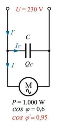
$$Q_c = P(\text{tg } \varphi - \text{tg } \varphi') = 1.000(\text{tg } 53^{\circ} - \text{tg } 18^{\circ}) = 1.002 \text{ VAR}$$
