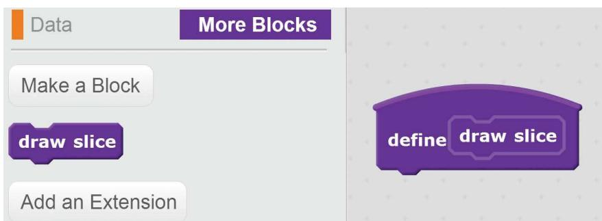
This new block with the curved top in the Scripts Area is the *defining* block for the **draw slice** block. When you want to use this new defining block, you must also drag the **draw slice** block, which is the *calling* block, from the Blocks Area into the code. Whenever Scratch runs this calling block, the code in the defining block is run.
