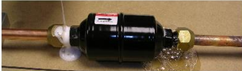
example of bubbling caused by leakage
