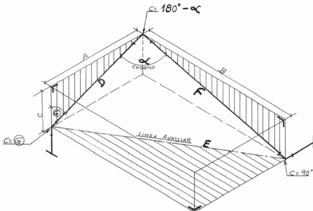
$$\left. \begin{array}{l} F = \sqrt{B^2 + C^2} \\ D = \sqrt{A^2 + C^2} \\ E = \sqrt{B^2 + A^2} \end{array} \right\} \quad \cos \alpha = \frac{D^2 + F^2 - E^2}{2 \cdot D \cdot F}$$
