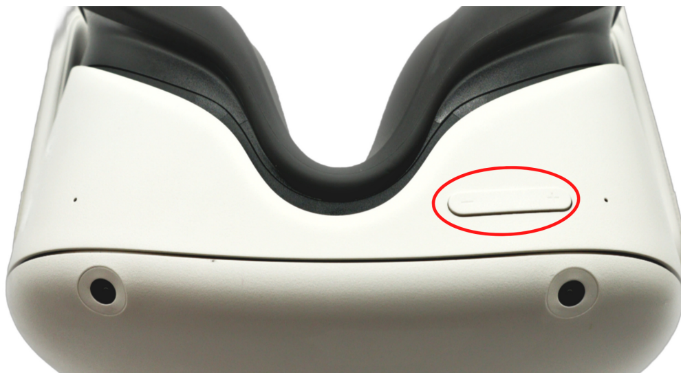
Fig. 5b. Volume buttons on underside of visor
