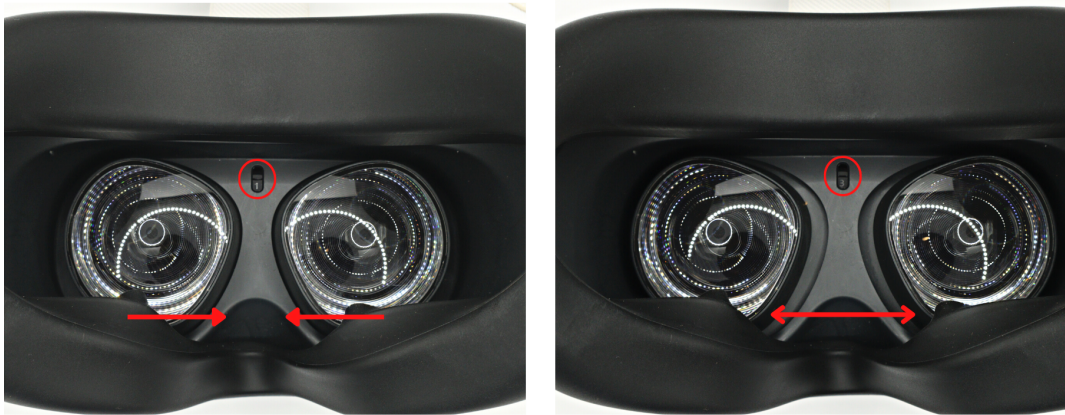
Fig. 5a. Lens-spacing slider inside visor
