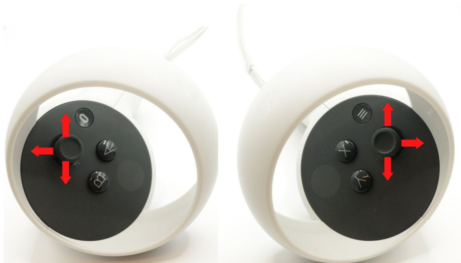
Fig. 4a. Controller analog sticks have 360-degree rotation
