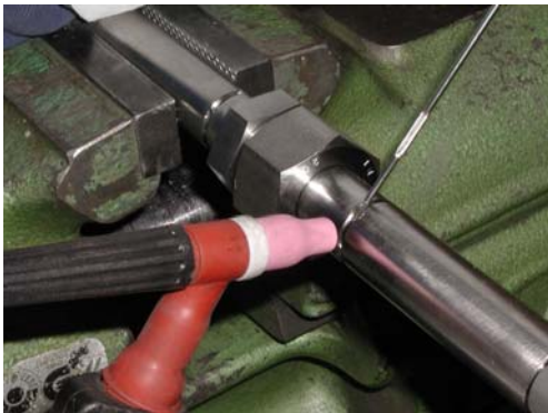
3. Tack-welding when bolted together. Clamping nut slightly tightened. Pay attention to the negative pole
