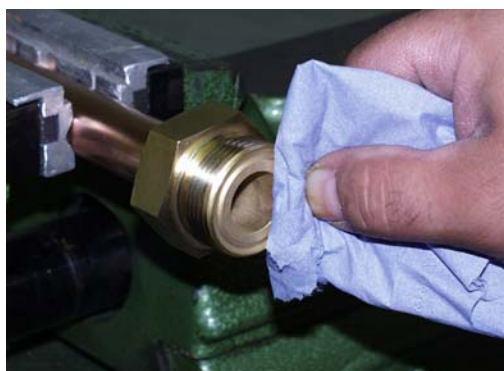
8. Before assembling clean the DILO tongue < and groove
