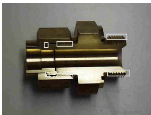
10. Lubricating points at a DILO tube union
