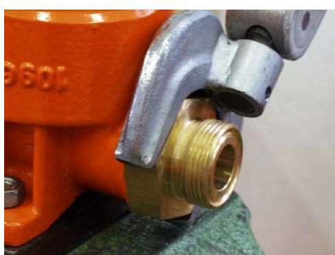
12. Sealing of the screwed plug between cage or block
