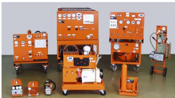
SF 6 -maintenance devices
