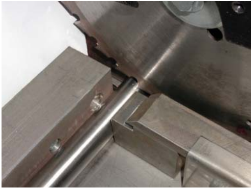
1. Saw off the tubes rectangularly
