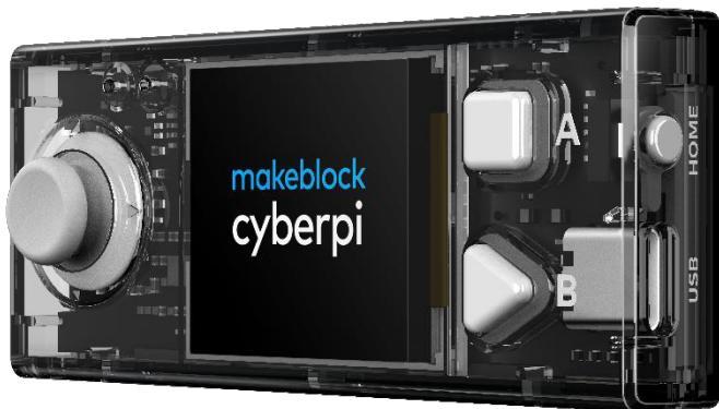
Mounted on the mBot2 there is a CyberPi. A CyberPi is a small, programmable microcomputer. You give the CyberPi commands using the code blocks in mBlock. The CyberPi passes these commands back to the mBot2. You can remove the CyberPi from the mBot2.
