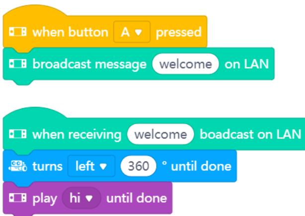
After uploading the programming codes, you must restart the mBot2 and/or CyberPi.
